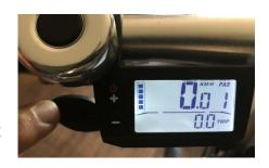
To engage the full assist mode using the throttle, simply begin moving the bike forward by pedaling, then press the thumb paddle forward, and you can stop pedaling. The bike needs to be moving forward before the full assist will engage; it will not take off on its own from a stand-still. This feature was designed as a safety measure.
